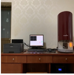
挪威Conoptica CU-10、CU-11激光测量 Norwegian Conoptica CU-10、CU-11 laser measuring instrument.
